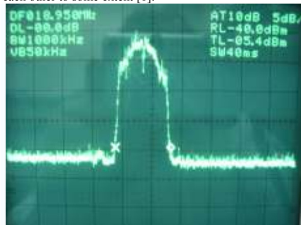
Figure 1. Spectral frequency bandwidth for 802.11g Access Point working on channel 8 (2.447GHz).
